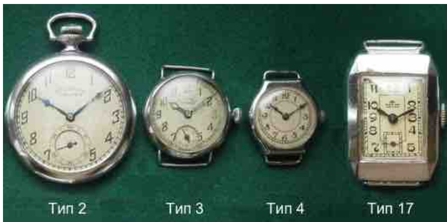
Types 2/3/4 have Hampden movements, the Type-2 being a 'Viking' movement, the Type-3 a No. "400" and an "8.0" movement in the Type-4. Courtesy of Alex Ballod.
